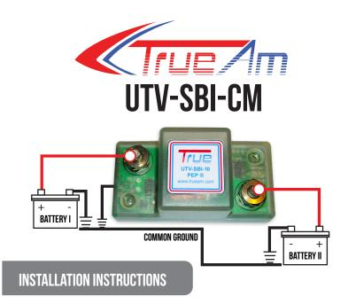
FYI: The SBI is designed ambidextrous so it cannot be installed backwards. Either stud can be connected to either battery's positive terminal.
